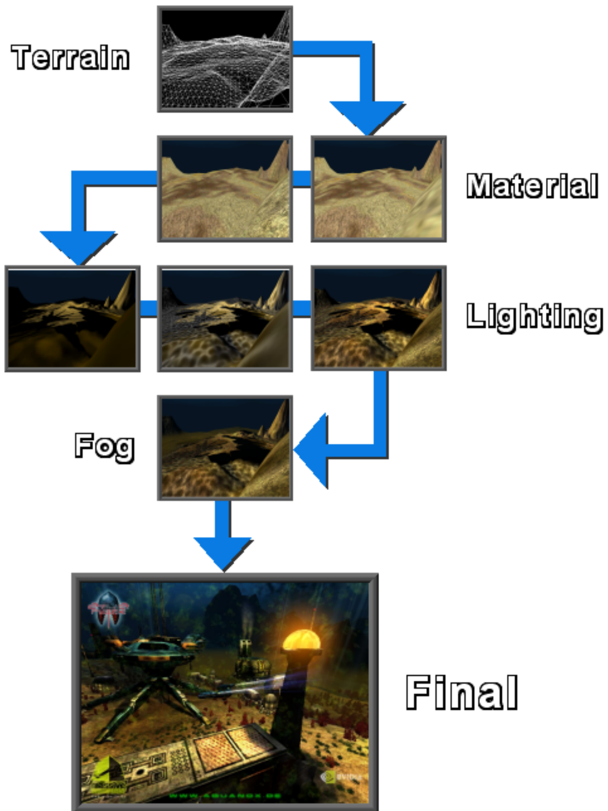
Figure 1: The main stages of the terrain rendering pipeline in the AquaNox game engine.
